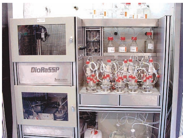
Figure 2. DioRaSSP Synthesizer: the first fully automated solution-phase peptide synthesizer.
